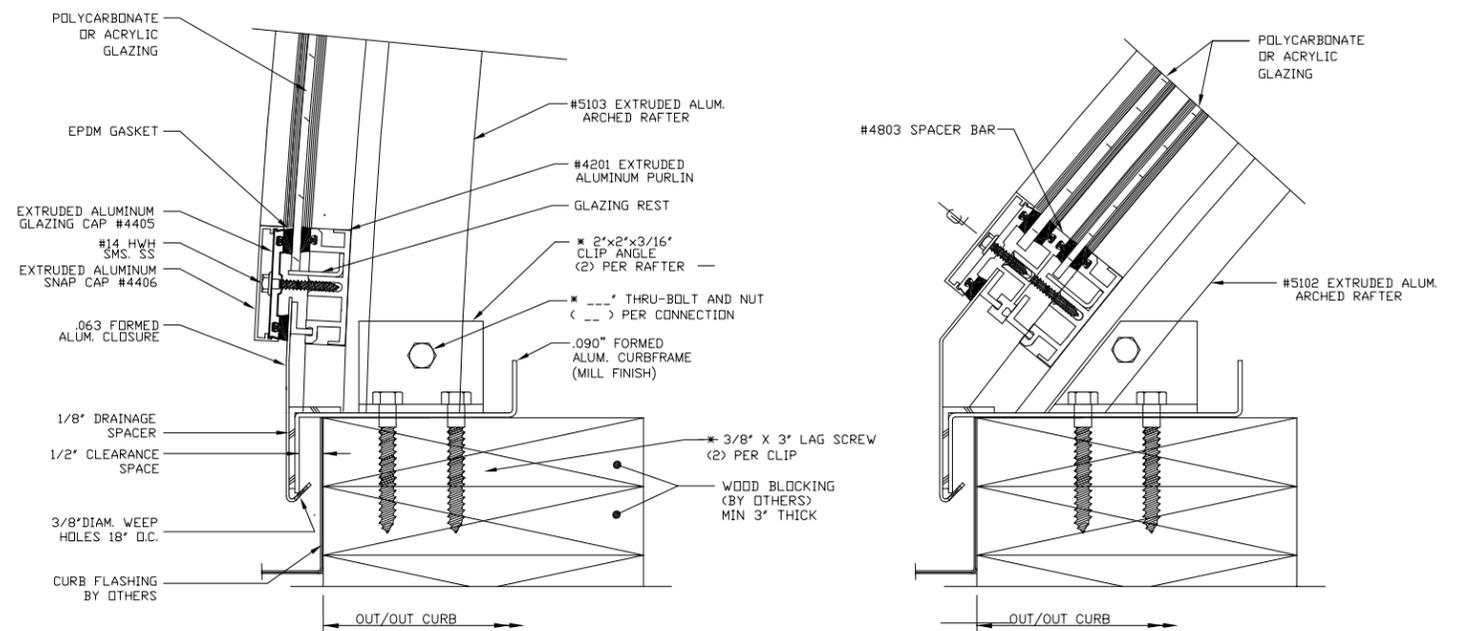
**O SINGLE GLAZED #5103 RAFTER CONNECTION TO CURB AT SILL OF 50% RISE VAULT**
